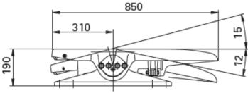
Suitable for 3½" king pins (G S) as per ECE R55-01, DIN 74083, ISO 4086 and steering wedges as per ECE R55-01, DIN 74085.
