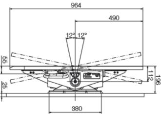
Suitable for  $3\frac{1}{2}$ " king pins (G S) as per ECE R55-01, DIN 74083, ISO 4086 and steering wedges as per ECE R55-01, DIN 74085.
