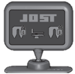
5th wheel open/ready for coupling
