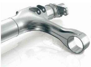
The compact axle beam gives the axle series the name DCA – Durable Compact Axle. Integrating all the axle functions creates a compact axle housing that is extremely durable and lightweight thanks to its innovative design. The axle housing integrates the trailing arm, axle tube, brake flange and axle journal, forming a perfect unit.
