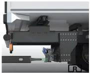
With the aid of the crosshair, the driver can aim for the towing eye, making it easier to drive towards the middle of the trailer. The green lines indicate the optimum coupling height.
